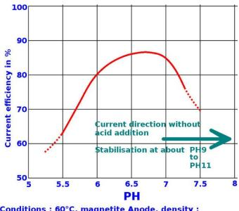
Conditions : 60°C, magnetite Anode, density : 30mA/Cm<sup>2</sup>, NaCl : 230g/L, 2g/L Sodium Dichromate. From Journal of Electrochemical Technology 6 (1968) 402
