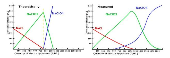
We can seen that the formation of perchlorate is not simultaneous with the disappearance of NaCl. With years of experience, I can say that my right graph is a bit exaggerated : the moment apparition of violet under the drop of methylene blue correspond to the end of chloride very closed to 0%, I'll confirm that point with measure test in a future.
