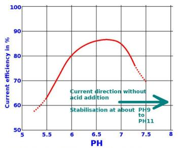
Conditions : 60°C, magnetite Anode, density : 30mA/Cm², NaCl : 230g/L, 2g/L Sodium Dichromate. From Journal of Electrochemical Technology 6 (1968) 402
